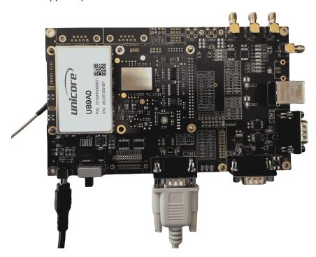
3. Select a GNSS antenna with appropriate gain, fix it in a stable, interference-free, and non-occluded area, and use the appropriate cable to connect the antenna with UB9A0 ANT interface.
